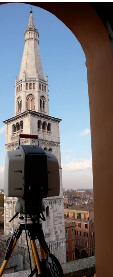
Torre Ghirlandina e strumento laser scanner (laser scanner terrestre HDS Scanstation2 della Leica Geosystems). Ghirlandina Tower and laser scanner instrument (HDS Scanstation2 terrestrial laser scanner from Leica Geosystems).
